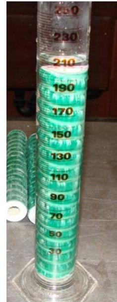
Figure 21: Test pieces with hollow section and measuring cup.
