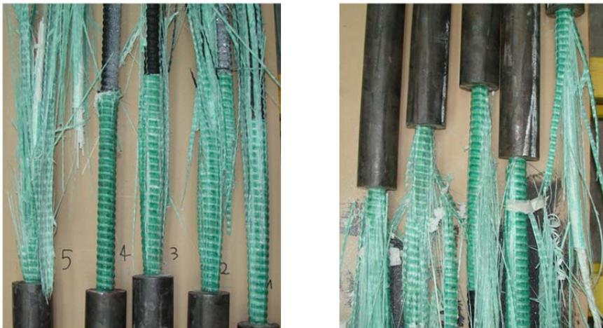
Figure 5: Photograph of failure patterns. The black color was applied for the image correlation measurements.
