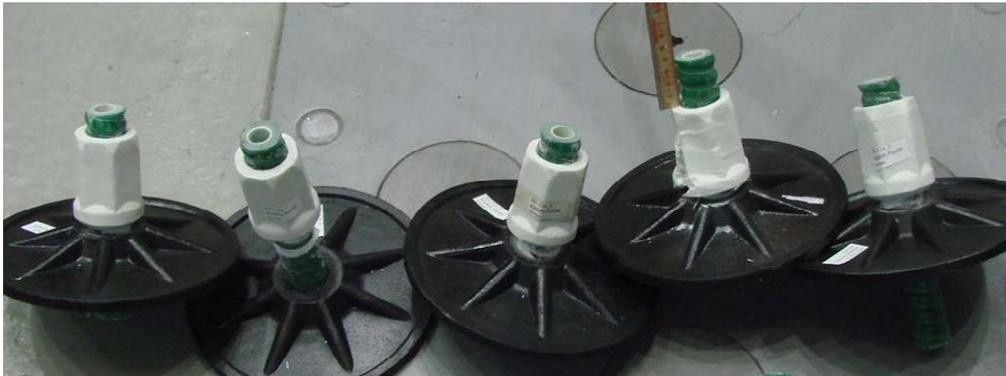
Figure 10: GRP Nuts and plates after the test. Since the nuts could not be loosened, the bolts were cut after the tests.
