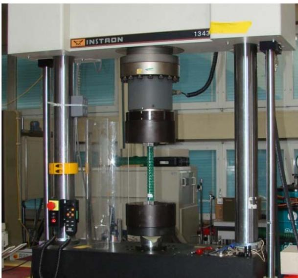
Figure 17: Torsion test machine with clamped test piece prior to the test.
