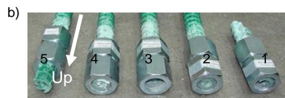
Figure 11: Steel Nuts after the tests. a) L = 1 x 45 mm and b) L = 2 x 45 mm. Since the nuts could not be loosened, the bolts were cut after the tests.
