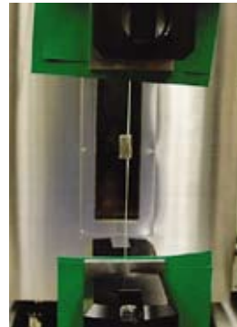
Photo 2: Tensile testing of a BarChip strand
