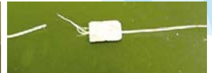
Photo 3: BarChip fibre strand after testing
