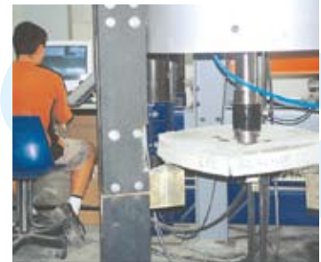
Steel Fibre: 54.4% Retention of Energy Absorption
