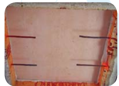
Specimen Containing 1.5Kg/m 3 BarChip F
